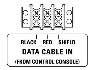
You may purchase data cable from the factory, or you may source it elsewhere. We recommend (and supply) cable that is rated for direct burial. It includes two insulated 22 AWG stranded conductors (red and black), along with a non-insulated conductor, all wrapped by a braided or foil shield. This document will discuss, in a few pages, what the other end of this cable is connected to.
